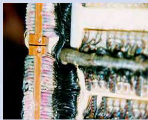
Communication panel aboard the Mir Space Station which lost function due to biodegradation by a fungal contaminant.
